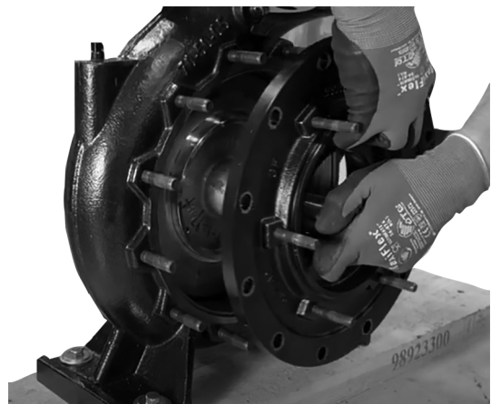
20. Remove pump cover and the impeller.
