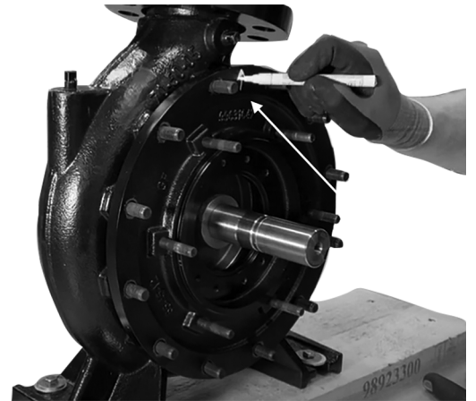
20. Remove pump cover and the impeller.
