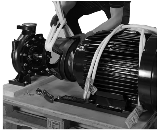
18. Loosen pump cover from pump housing.
