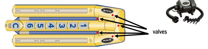
**IMPORTANT**: Inflate tubes only until the Super Shuttle takes shape (about 80% to 90% air volume).
