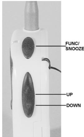
**Snooze/Function** – This is a push button that switches between time, date and temperature display and alert message area. By pressing and holding this button you can switch between alert with siren voice and alert message, alert message only, turn the weather alert off or listen to the weather broadcast.
