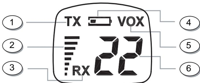
1. **TRANSMIT (TX) ICON** – Indicates radio is transmitting a signal.
