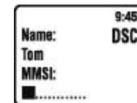
Write the identification code using the alphanumerical keypad (obligatorily 9 digits)
