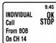
pressure to the function key "STOP" will deactivate the alarm.
