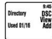
5. By pressing the function key “Add” you will have the possibility to add further MMSI addresses. Pressing the function key “VIEW” you will have the possibility to modify/cancel the address shown on the display.
