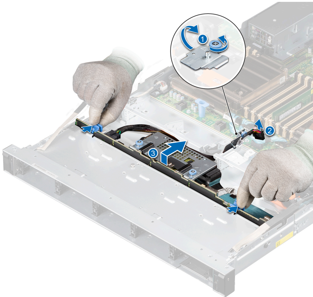
Figure 55. Removing the drive backplane
