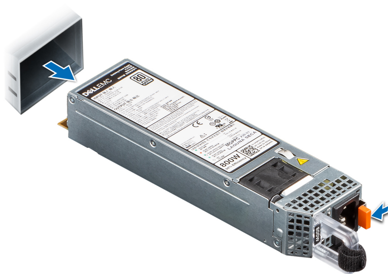
Figure 132. Removing a power supply unit
