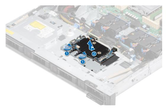
Figure 111. Removing the front mounting front PERC module
