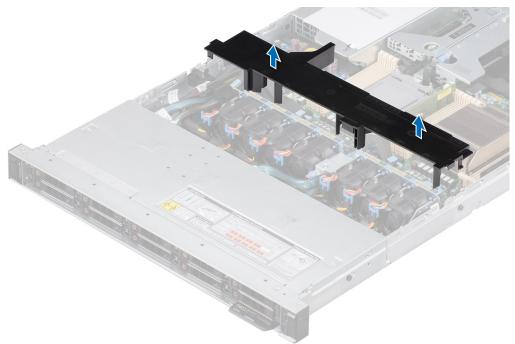
Figure 18. Removing the air shroud
