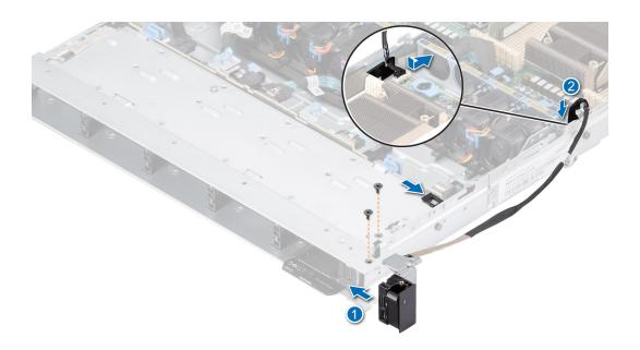
Figure 131. Installing the right control panel
