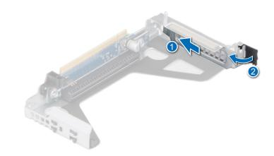
Figure 81. Installing filler bracket in the Riser 1
