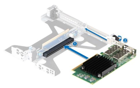
Figure 92. Installing an expansion card into a Riser 2c
