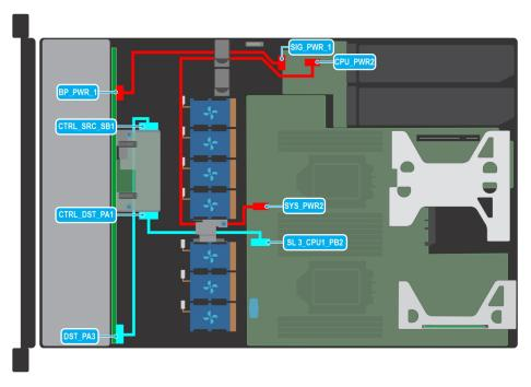
Figure 41. Cable routing - 10 x 2.5-inch drive SAS/SATA backplane with fPERC, Butterfly riser
