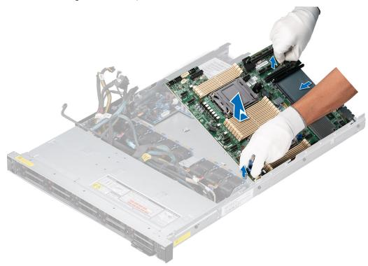
Figure 125. Removing the system board
