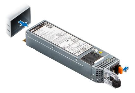
Figure 121. Removing a power supply unit
