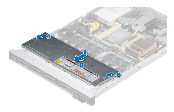
Figure 17. Installing the drive backplane cover
