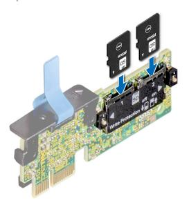
Figure 100. Installing the MicroSD card
