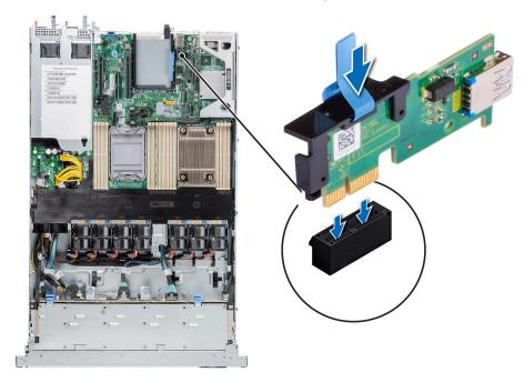
Figure 116. Installing the internal USB card
