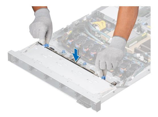
Figure 36. Installing the drive backplane
