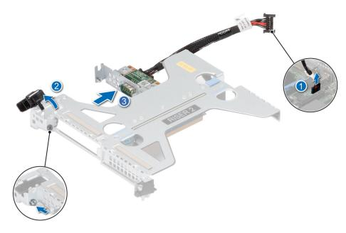
Figure 95. Removing the Serial COM port
