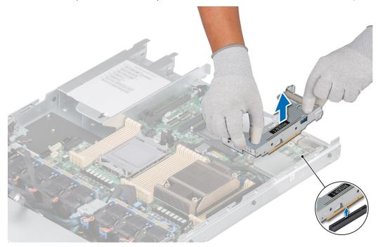
Figure 69. Removing the Riser 1
