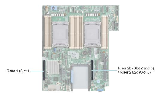
Figure 64. Expansion card slot connectors
