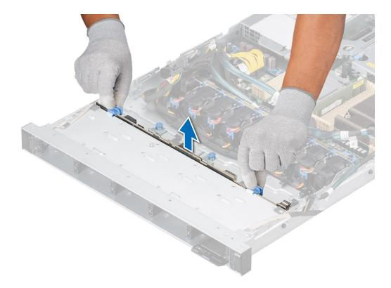
Figure 35. Removing the backplane
