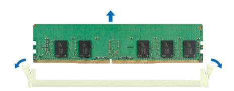
Figure 50. Removing a memory module
