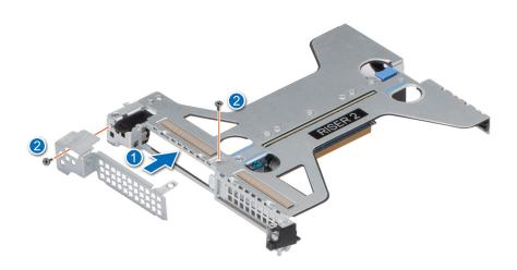
Figure 96. Installing the PCIe blank
