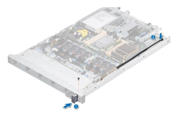
Figure 118. Installing the VGA module
