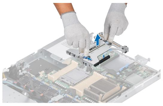
Figure 72. Removing the Riser 2c
