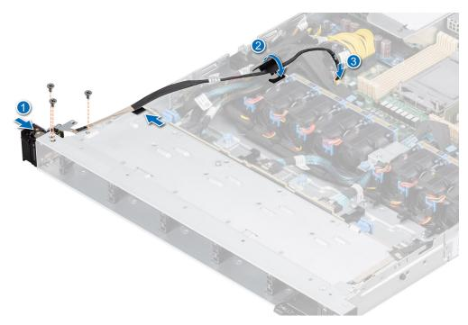
Figure 129. Installing the left control panel
