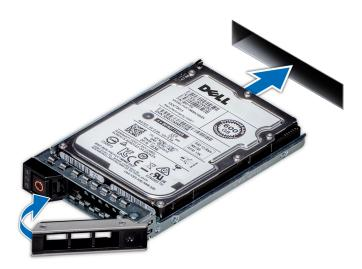
Figure 27. Installing a drive carrier
