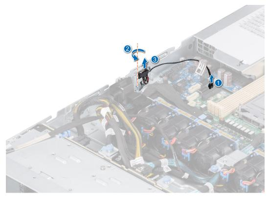
Figure 22. Removing the intrusion switch module
