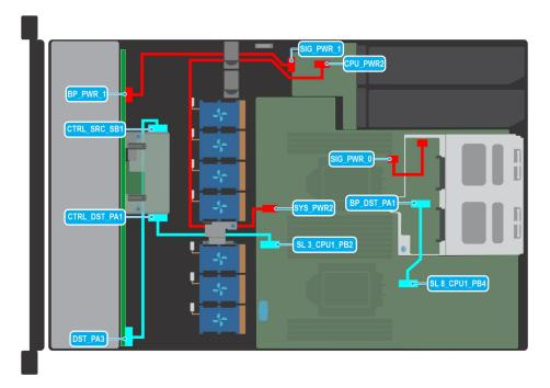
Figure 46. Cable routing -  $10 \times 2.5$ -inch drive SAS/SATA backplane with rear drive cage with NVMe backplane, Butterfly riser
