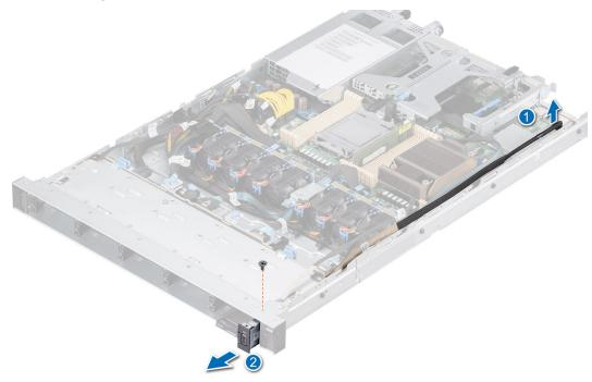
Figure 117. Removing the VGA module
