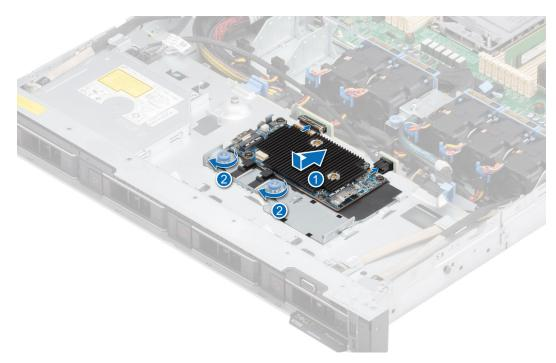
Figure 112. Installing the front mounting front PERC module
