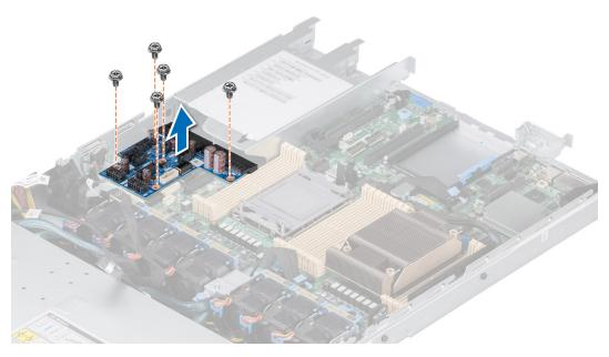
Figure 123. Removing the power interposer board
