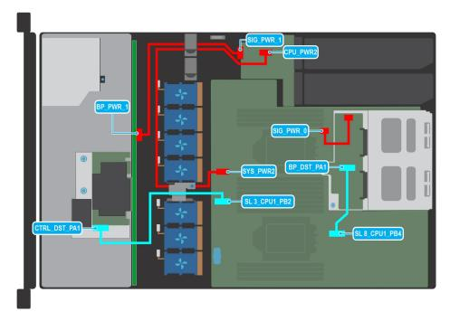
Figure 43. Cable routing -  $4 \times 3.5$ -inch drive SAS/SATA backplane wih fPERC with rear drive cage with NVMe backplane
