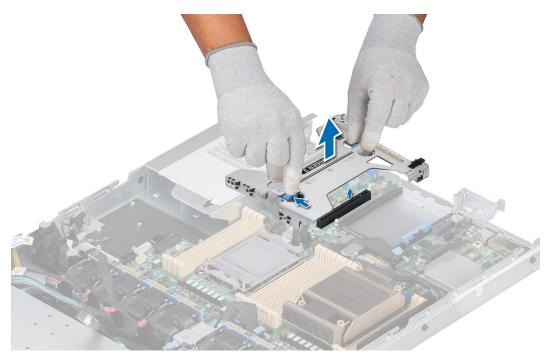
Figure 70. Removing the Riser 2a
