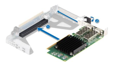
Figure 89. Installing an expansion card into a Riser 1
