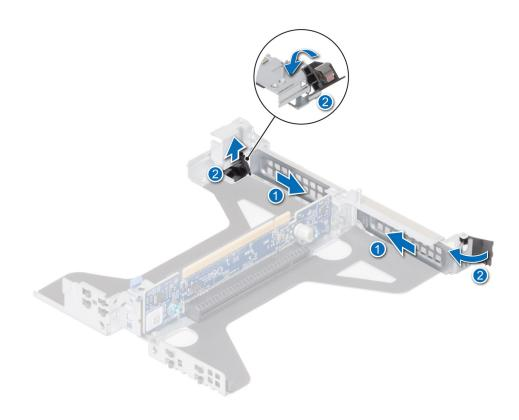
Figure 82. Installing filler bracket in the Riser 2a
