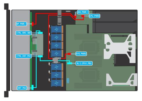
Figure 39. Cable routing -  $10 \times 2.5$ -inch drive backplane with Butterfly riser and fPERC
