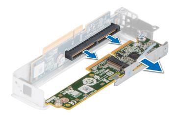
Figure 103. Removing the M.2 BOSS card from the M.2 BOSS riser
