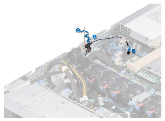
Figure 23. Installing the intrusion switch
