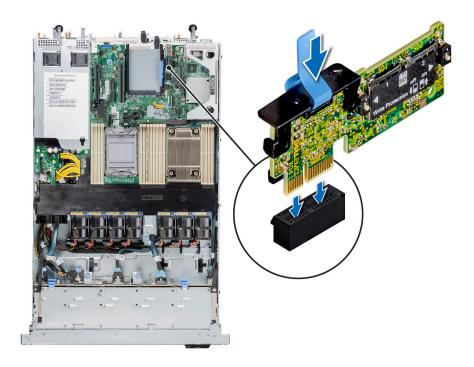
Figure 108. Installing the IDSDM module
