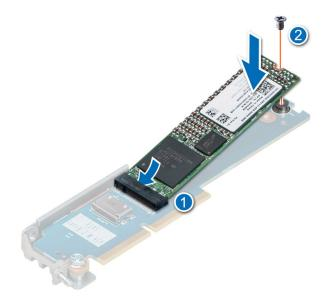
Figure 106. Installing the M.2 SSD module
