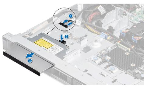
Figure 30. Removing the optical drive
