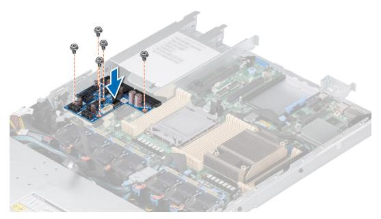
Figure 124. Installing the power interposer board
