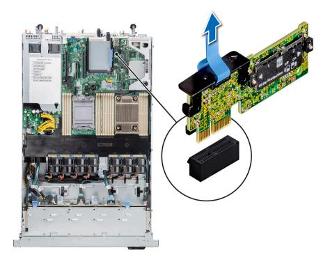
Figure 107. Removing the IDSDM module
