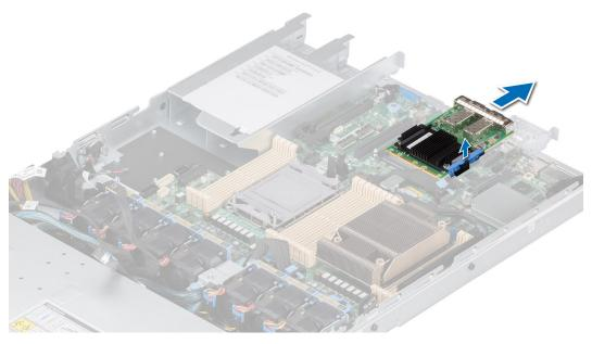
Figure 109. Removing the OCP card
