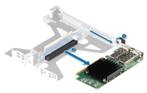
Figure 80. Removing an expansion card from Riser 2c
