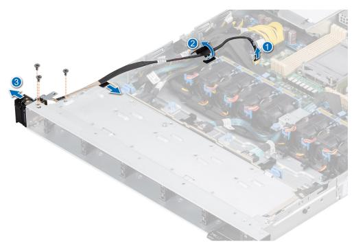
Figure 128. Removing the left control panel
