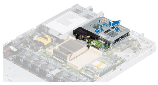
Figure 94. Installing the 2.5-inch rear drive cage
