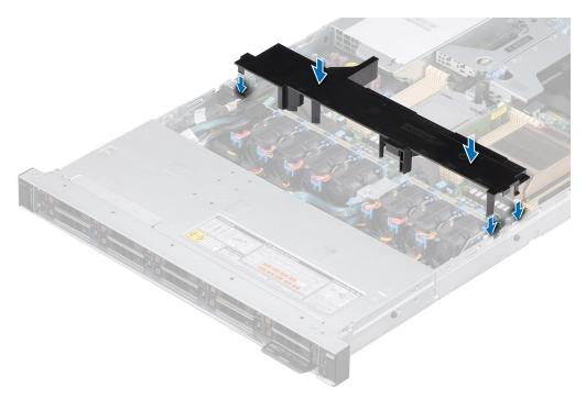
Figure 19. Installing the air shroud
