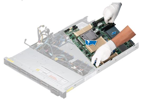
Figure 126. Installing the system board
