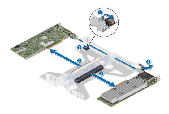
Figure 78. Removing an expansion card from Riser 2a
