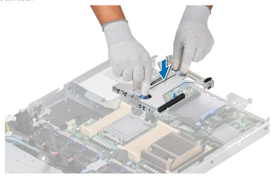
Figure 74. Installing the Riser 2a
