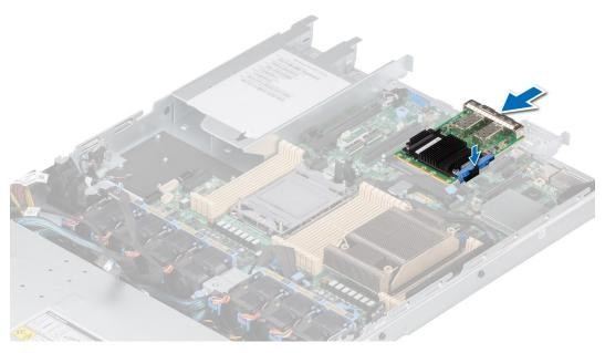
Figure 110. Installing the OCP card
