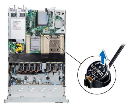
Figure 113. Removing the system battery
