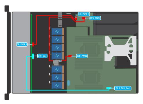
Figure 37. Cable routing - 4 x 3.5-inch drive backplane with Butterfly riser
