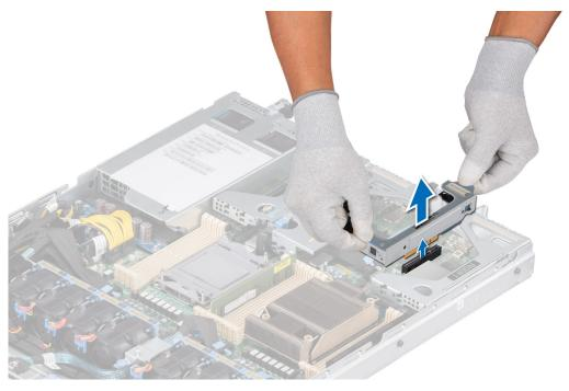
Figure 101. Removing the M.2 BOSS riser
