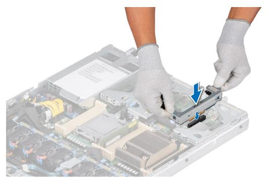
Figure 102. Installing the M.2 BOSS riser
