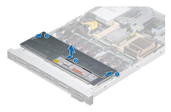
Figure 16. Removing the drive backplane cover
