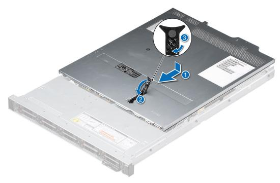
Figure 15. Installing the system cover
