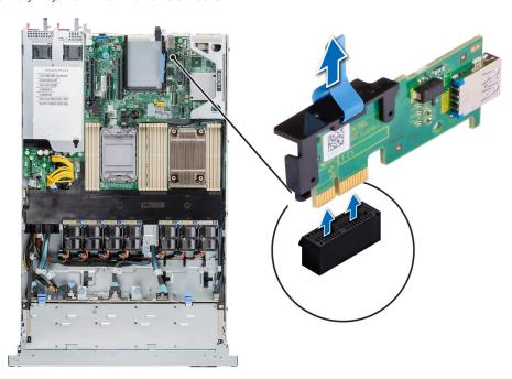
Figure 115. Removing the internal USB card
