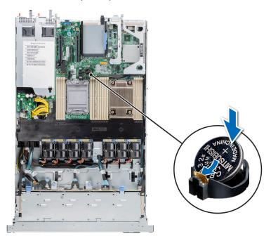
Figure 114. Installing the system battery
