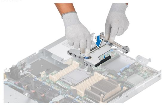
Figure 76. Installing the Riser 2c
