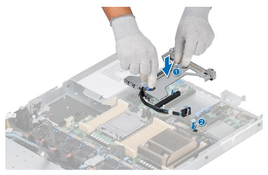
Figure 75. Installing the Riser 2b with SNAPI module
