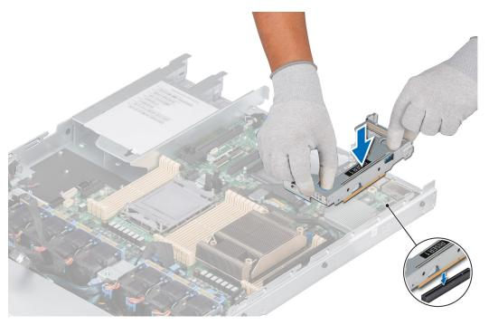
Figure 73. Installing the Riser 1
