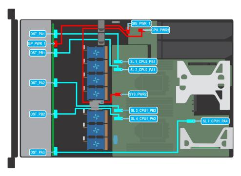
Figure 40. Cable routing -  $10 \times 2.5$ -inch drive backplane on the onboard controller (4:6 NVMe)
