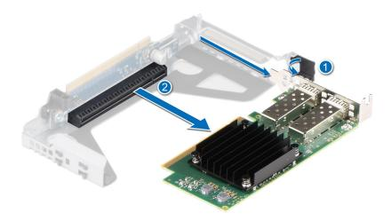
Figure 77. Removing an expansion card from the Riser 1
