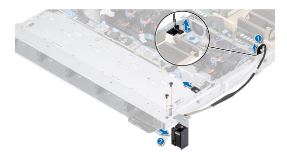
Figure 130. Removing the right control panel
