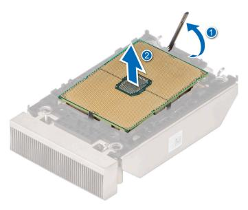
Figure 54. Lift the TIM break lever
