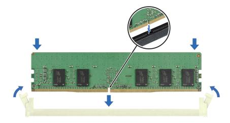
Figure 51. Installing a memory module
