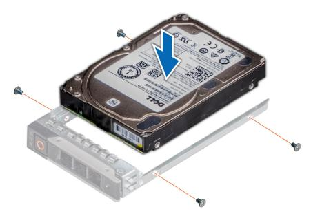
Figure 29. Installing a drive into the drive carrier
