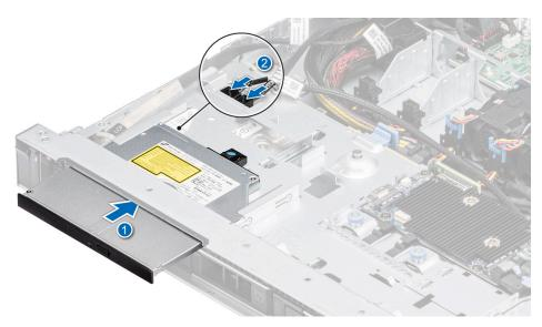
Figure 31. Installing the optical drive
