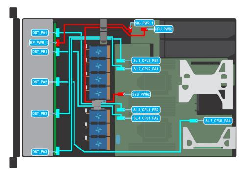
Figure 38. Cable routing -  $10 \times 2.5$ -inch drive backplane to the onboard controller (6:4 NVMe)
