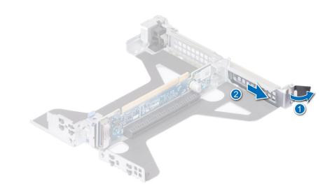
Figure 87. Removing filler bracket from Riser 2b (SNAPI)
