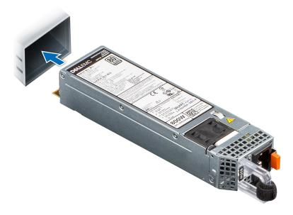
Figure 122. Installing a power supply unit
