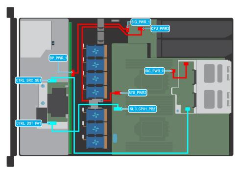
Figure 44. Cable routing -  $4 \times 3.5$ -inch drive SAS/SATA backplane with rear drive cage with SAS backplane, Butterfly riser
