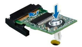
Figure 127. Installing the TPM
