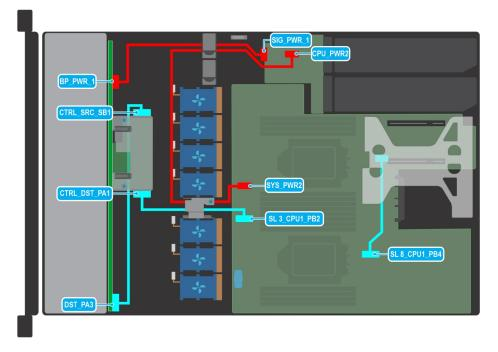
Figure 45. Cable routing -  $10 \times 2.5$ -inch drive SAS/SATA backplane with Butterfly riser
