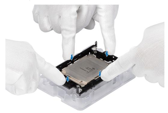
Figure 58. Press the carrier on the four sides
