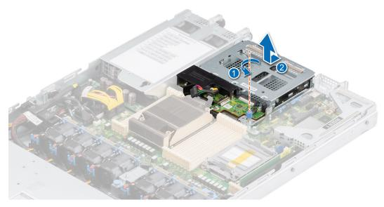
Figure 93. Removing the 2.5-inch rear drive cage
