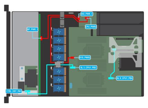
Figure 47. Cable routing - 8  $\times$  2.5-inch drive SAS/SATA backplane with SNAPI riser
