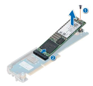
Figure 105. Removing the M.2 SSD module
