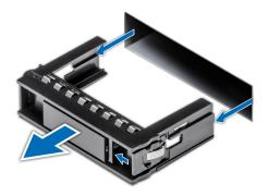
Figure 24. Removing a drive blank
