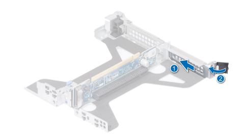
Figure 83. Installing filler bracket in the Riser 2b (SNAPI)
