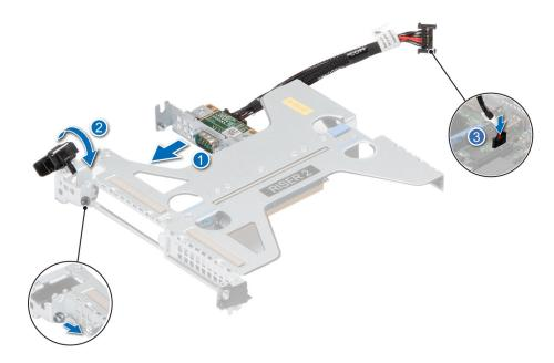
Figure 98. Installing the Serial COM port
