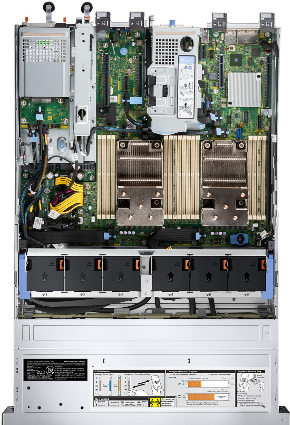
Figure 15. Inside the 12 x 3.5-inch system
