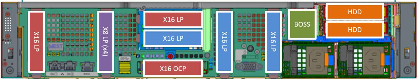
Figure 10. Rear view of the system
