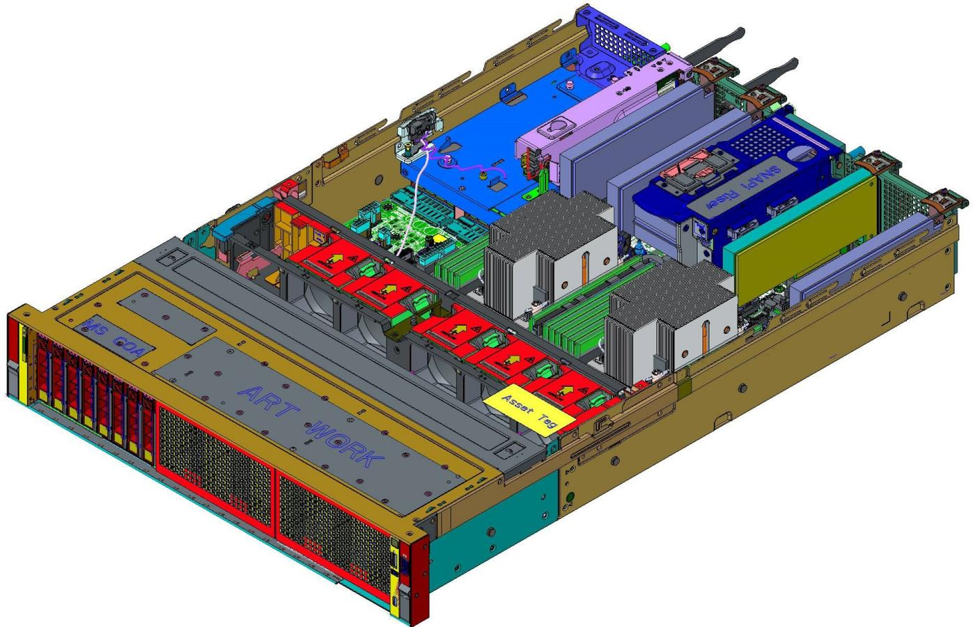
Figure 13. Inside the 8 x 2.5-inch system
