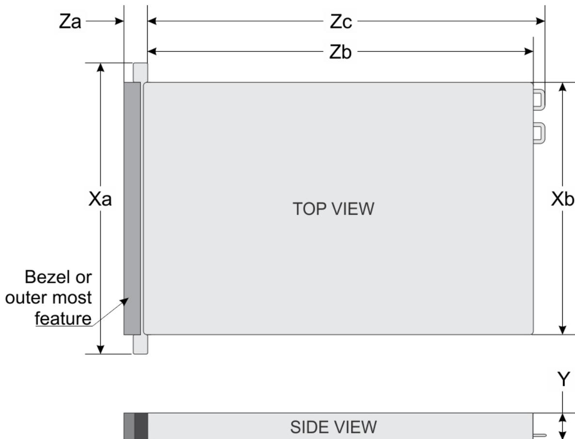
Figure 31. PowerEdge R750xs chassis dimensions
