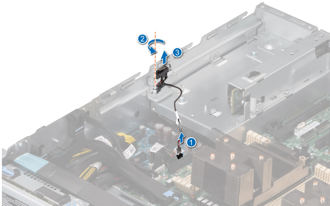
Figure 35. Removing the intrusion switch module
