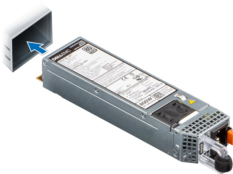
Figure 123. Installing a power supply unit
