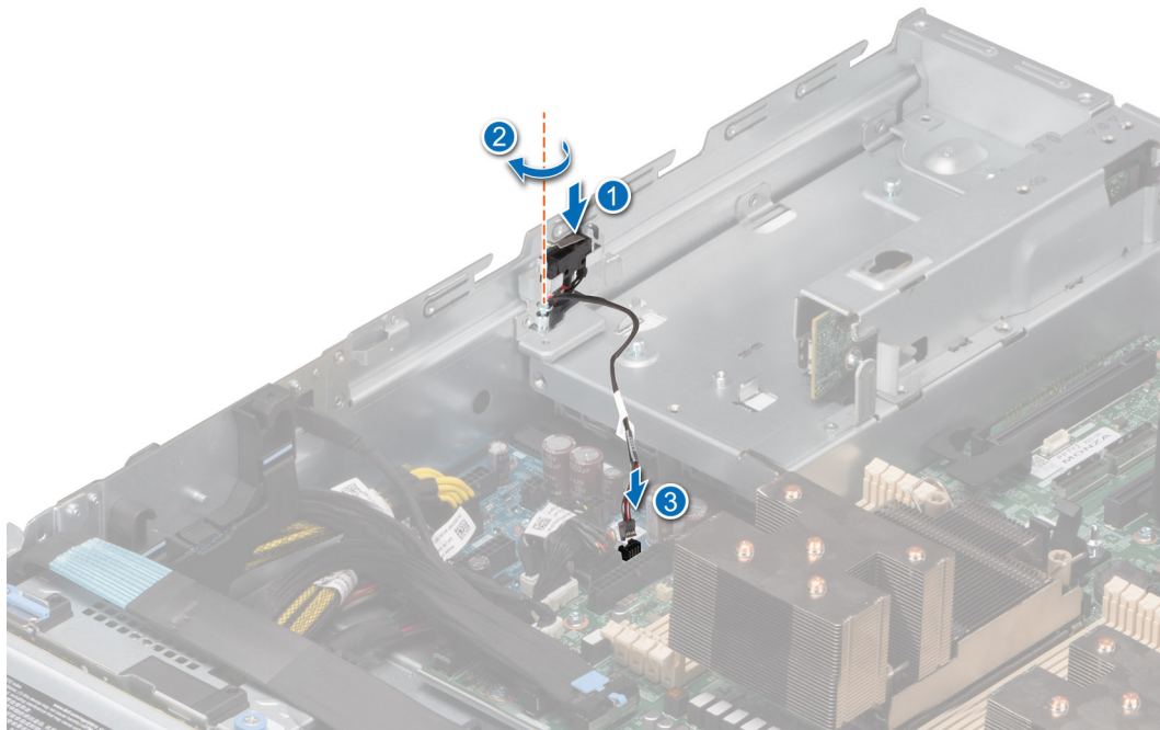
Figure 36. Installing the intrusion switch
