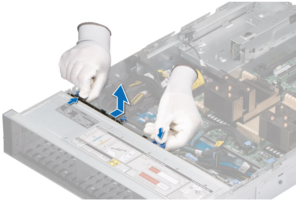
Figure 49. Removing the drive backplane
