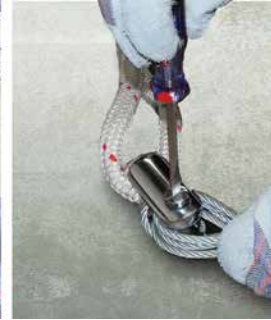
Replace and tighten pin
