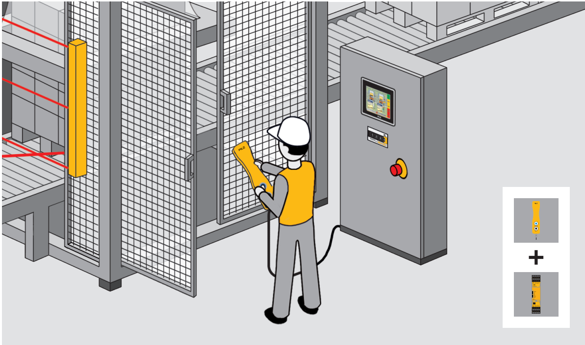
The optimum solution: two-hand monitoring with the manually operated control device PITjog and the safety relay PNOZ s6.
