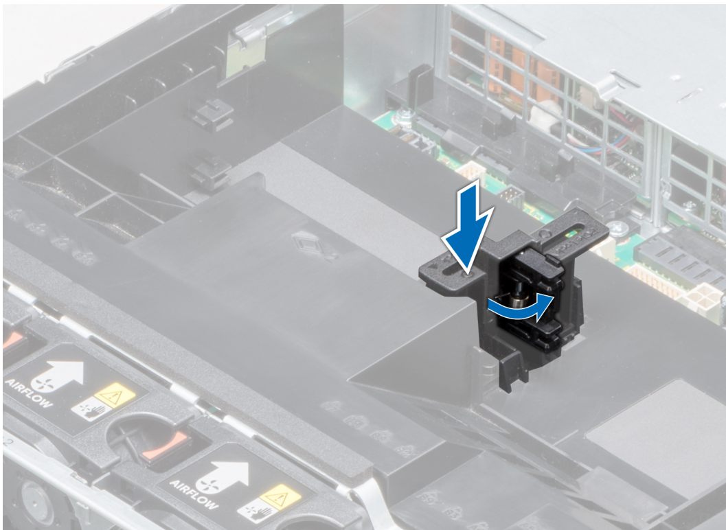
Figure 64. Opening the PCIe card holder latch
