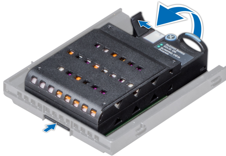
Figure 43. Removing NVDIMM-N battery from the bracket
