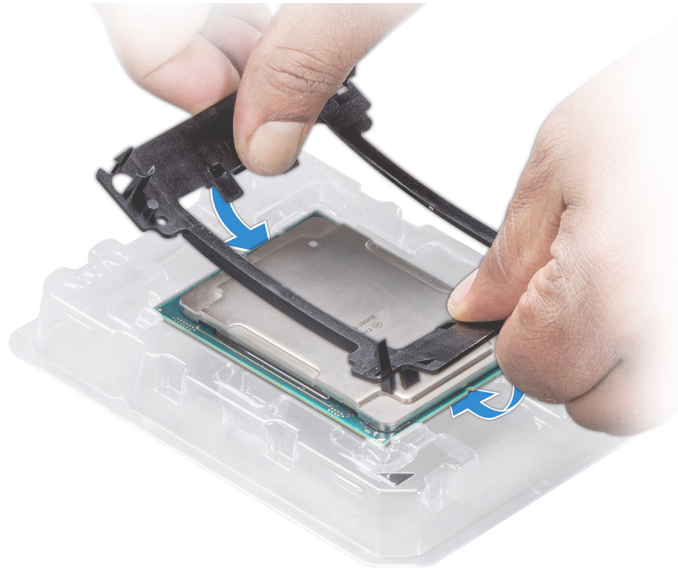
Figure 60. Installing the processor bracket
