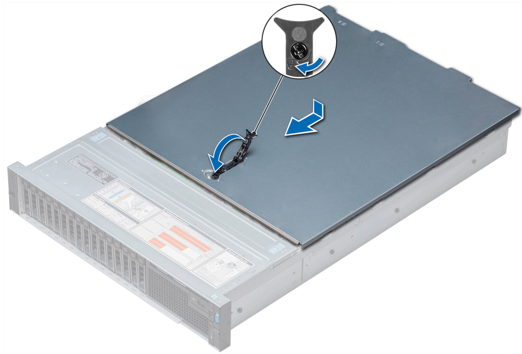
Figure 26. Installing system cover
