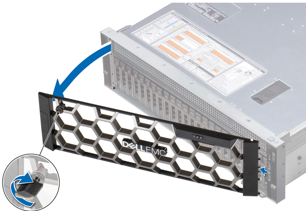
Figure 20. Removing the optional front bezel with the LCD panel
