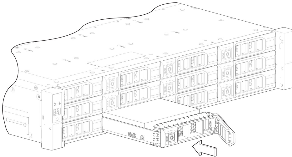
Figure 41. Installing an LFF drive carrier module (1 of 2)
