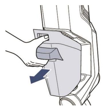
• Remove strainer from tank and discard debris
