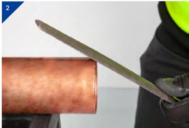
2. Carefully deburr and wipe clean the end of the tube Internally.
