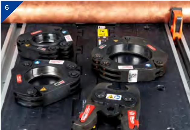
6. Select the appropriate sized collar, check it is clean and that the surface of the pressing area is smooth.
