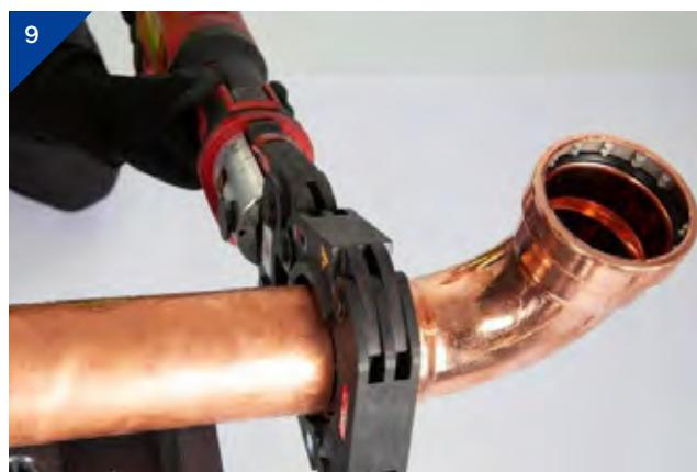
9. Open the adaptor jaw by depressing the jaw levers and attach to the press collar so that the claws of the jaw grip around the pins of the press collar. Initiate the pressing job by pressing the start button.
