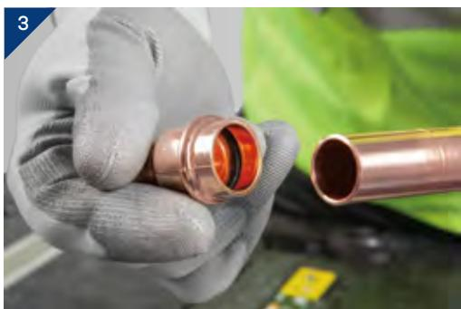
3. Check the Fitting and Tube End: Before inserting the tube, check that the body of the fitting is free from any physical damage, and check that the sealing element is clean, and seated in the groove; ensure that the tube end is not bent or damaged and is thoroughly deburred.
