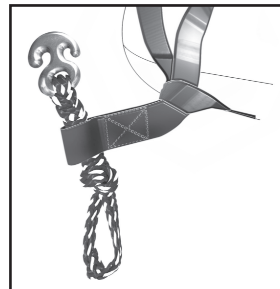
1: Locate the loop on the towable tow strap that is sewn to the towable. Put the 4K EZ Tow Aluminum Connector through the towable strap loop as shown above.
