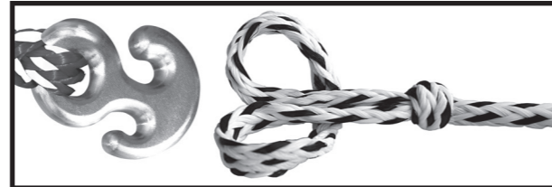
2: Take the tow rope put the end of the loop under itself, back towards the knot
