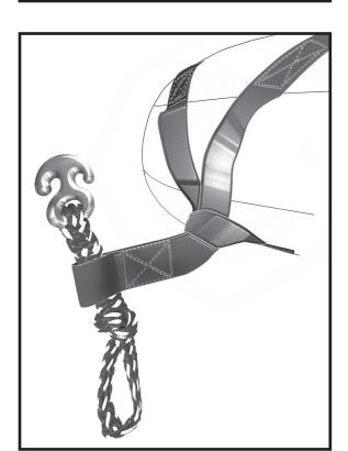
**1:** Locate the loop on the towable tow strap that is sewn to the towable. Put the 4K EZ Tow Aluminum Connector through the towable strap loop as shown above.
