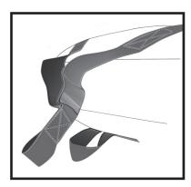
1: TOW SYSTEM. Put the top tow strap down through the bottom loop strap that is sewn to the bottom of the product.
