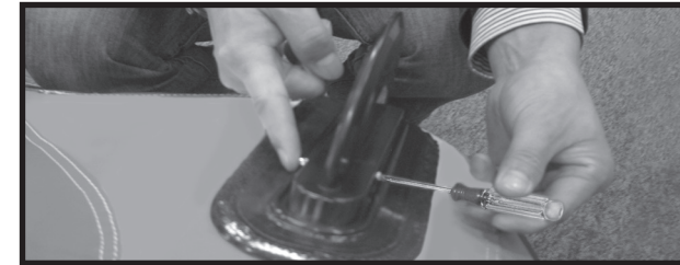
C3: After Sliding all your REMOVABLE SLALOM SPIN TECH FINS into all brackets place the bolts through all holes in each fin and bracket and hand tighten screws to the nut bolts.
