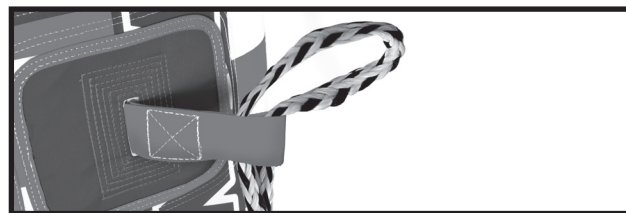
B2: Loop the 2K Tow Rope through and around the STATIC TOW SYSTEM loop as shown above. Then locate the end of 2K Tow Rope.
