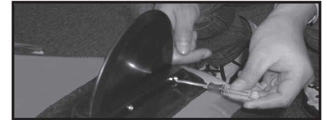
C4: Secure and tighten all screws on all fins and brackets.
