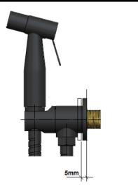
Wall plate tolerance of 5mm
