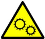
This symbol indicates the presence of moving parts inside the product that may present a pinch point if improperly contacted.
