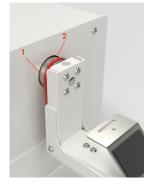
**4.** Keep tension on the orange belt (**1**) and push the arm downwards onto the driveshaft (**2**).
