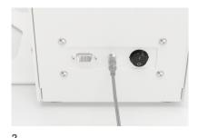
**2.** Turn the power switch located on the rear of the device to the **"ON"** position.
