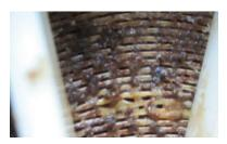
Photo of colloidal contamination
