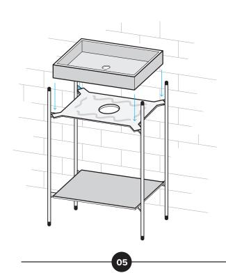
Apply glue to top base plate and carefully place sink on top.
