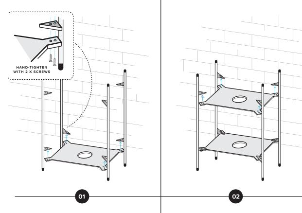
Ensuring base plate is positioned beneath pole tabs, hand tighten each corner with screws to secure position. Allow for some wiggle room. Repeat this process with second base plate. Once screws are hand-tightened, repeat tighten all screws with allen key.
