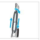
3. Wrap cord. To easily unwrap, turn Quick Release™ Cord Wrap down.
