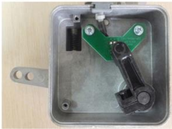
Picture 9 the position when motor stop running
