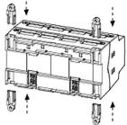
b) Place ECA500-II over a flat surface panel and mount it using(2) #8 x 1/2" screws
