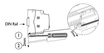
b) With screwdriveratposition (2) pull out ECA500-11 from DIN Rail as shown in figure.
