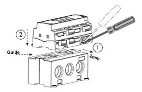
From Alignment Mark, move ECA500-11 relay towards, the left sliding through rail guide until it does Click, as shown in following picture:
