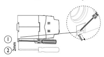
b) With screwdriver at position (2) pull out ECA500-11 from DIN Rail as shown in figure.
