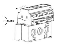
c) Insert both CT Input Terminals connecting ECA500-11 and CT Box.
