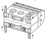
b) Place ECA500-II over a flat surface panel and mount it using(2) #8 x 1/2" screws
