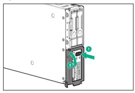
**2.** Install the server. When seated properly, the server will be flush with the front of the chassis and the release lever will close completely without resistance.
