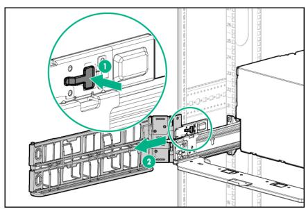
2. Move the cable management arm to the right rack rail and align the tab for opposite side mounting.
