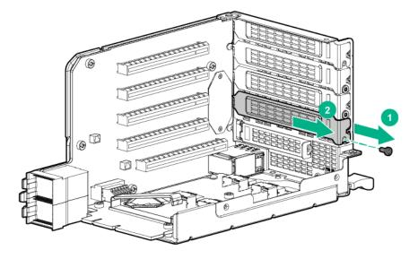
**4.** Install a supported expansion board option in one of the PCle expansion slots.
