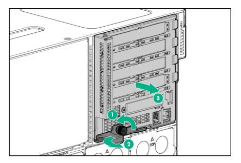
2. Remove the I/O module access panel.
