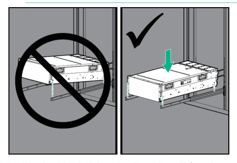
3. Install the chassis into the J-slot on the rails, and then pull it forward.
