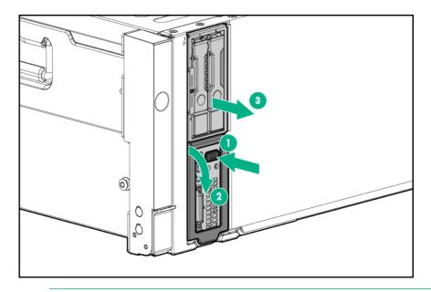
**CAUTION:** To avoid damage to the device, do not use the removal handle to carry it.
