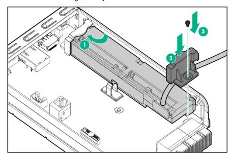
2. Connect the Smart Storage Battery cable to the Smart Storage Battery connector.
