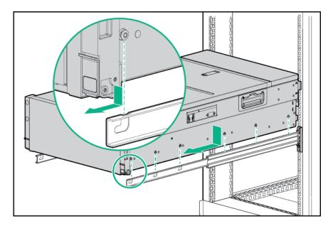
4. Press the Push tabs on each rail, and then slide the chassis into the rack. When the chassis stops midway, press the push tabs on each rail to release the chassis and slide it fully into the rack.
