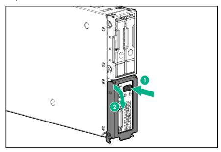
**2.** Install the server. When seated properly, the server will be flush with the front of the chassis and the release lever will close completely without resistance.
