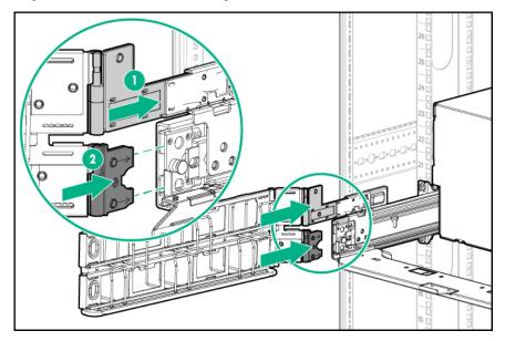
3. Press the latch and slide the cable management arm into place.
