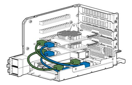
Dual-board option (I/O module with the x16 riser option)
