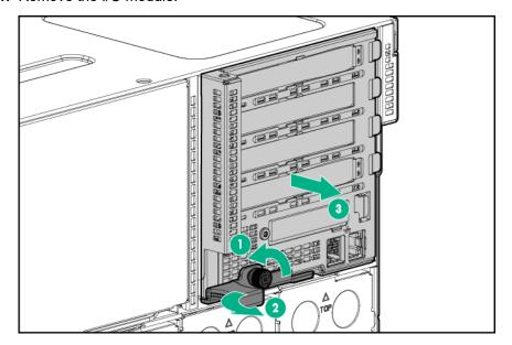
2. Remove the I/O module access panel.
