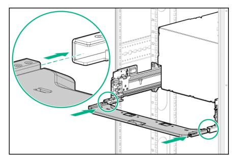
2. Align and install the cable management arm.
