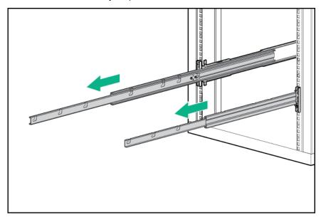
2. Fully extend the rails by pressing the push tabs and extending the rails until the rails click two times.
