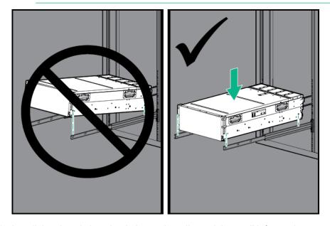
3. Install the chassis into the J-slot on the rails, and then pull it forward.
