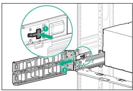
2. Move the cable management arm to the right rack rail and align the tab for opposite side mounting.
