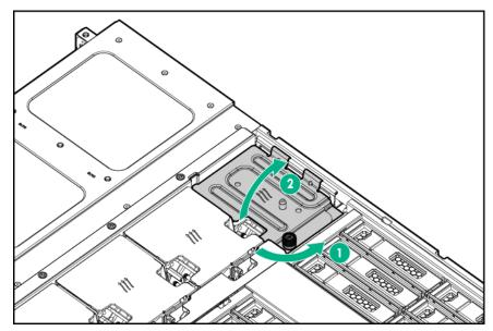
**b.** Remove the system fans from all 5 fan bays.
