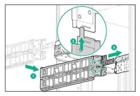
3. Align and install the cable management arm on the right rack rail.
