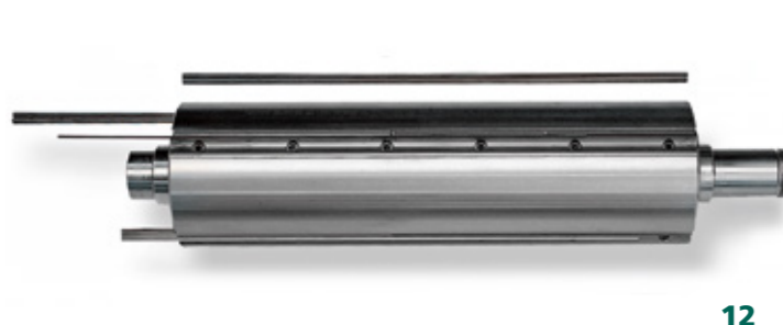
12 Monobloc planer shaft The mono-bloc planer shaft with disposable double-edge knives offers the following advantages: quick knife change, automatic locking with centrifugal force, precise positioning and assurance that knives remain locked when the machine is turned on.
