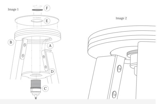
Before attaching your lampshade and lamp holder to the stand, you first need to attach the legs of the tripod to the plywood top plate.
