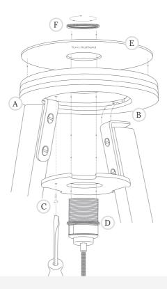
Before attaching your lampshade and lamp holder to the tripod, you first need to assemble the tripod stand and secure the legs in place using the locking disk and brass screw.
