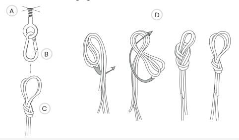
This product will hold a maximum weight of 100kg, however it must be hung from a suitable beam or joist capable of supporting at least 100kg plus the weight of Amble Hanging Seat (110.1kg).
