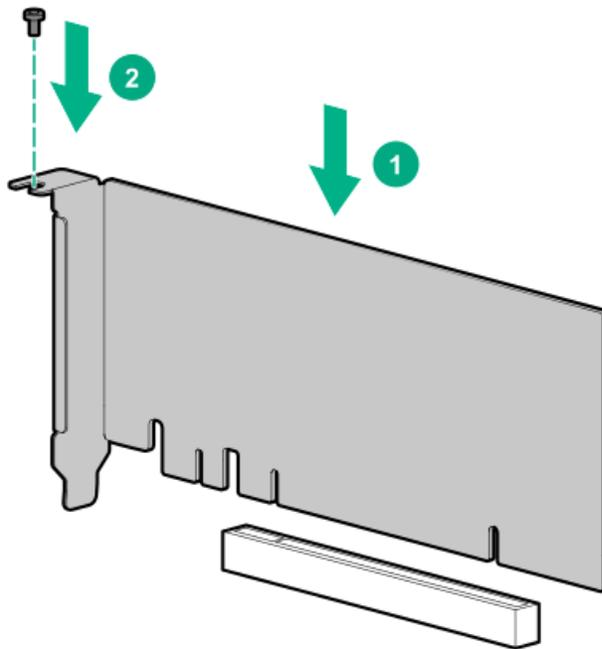
8. To install a full-height, half-length PCIe x16 expansion board, the two-slot PCIe riser cage option is required. To install an expansion board or type -p controller in this riser cage, do the following:
