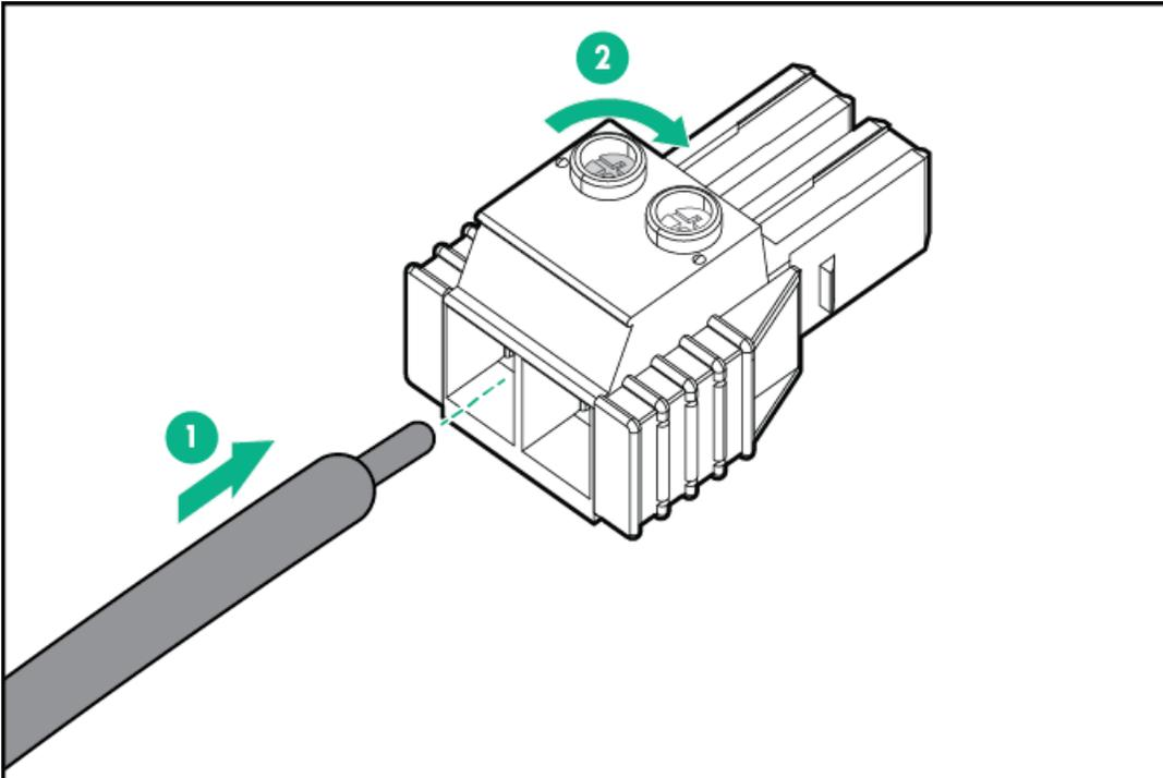
8. Insert the return wire into the right side of the connector, and then tighten the screw to 1.3 N m (10 lb-in) of torque.
