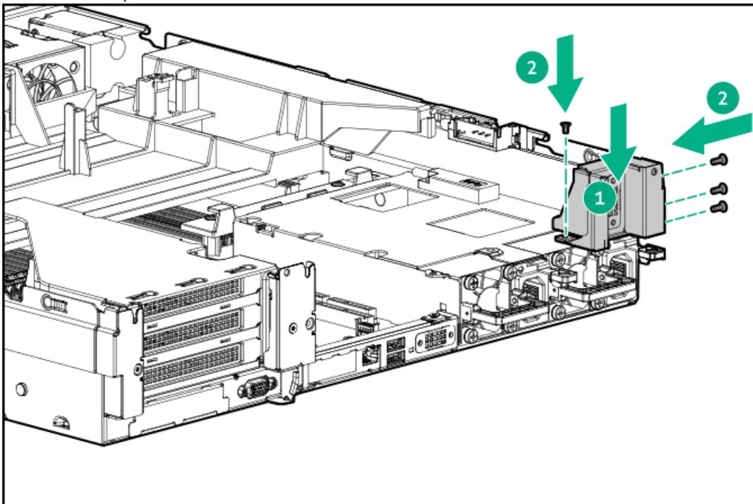
9. Install the PCIe riser cage.
