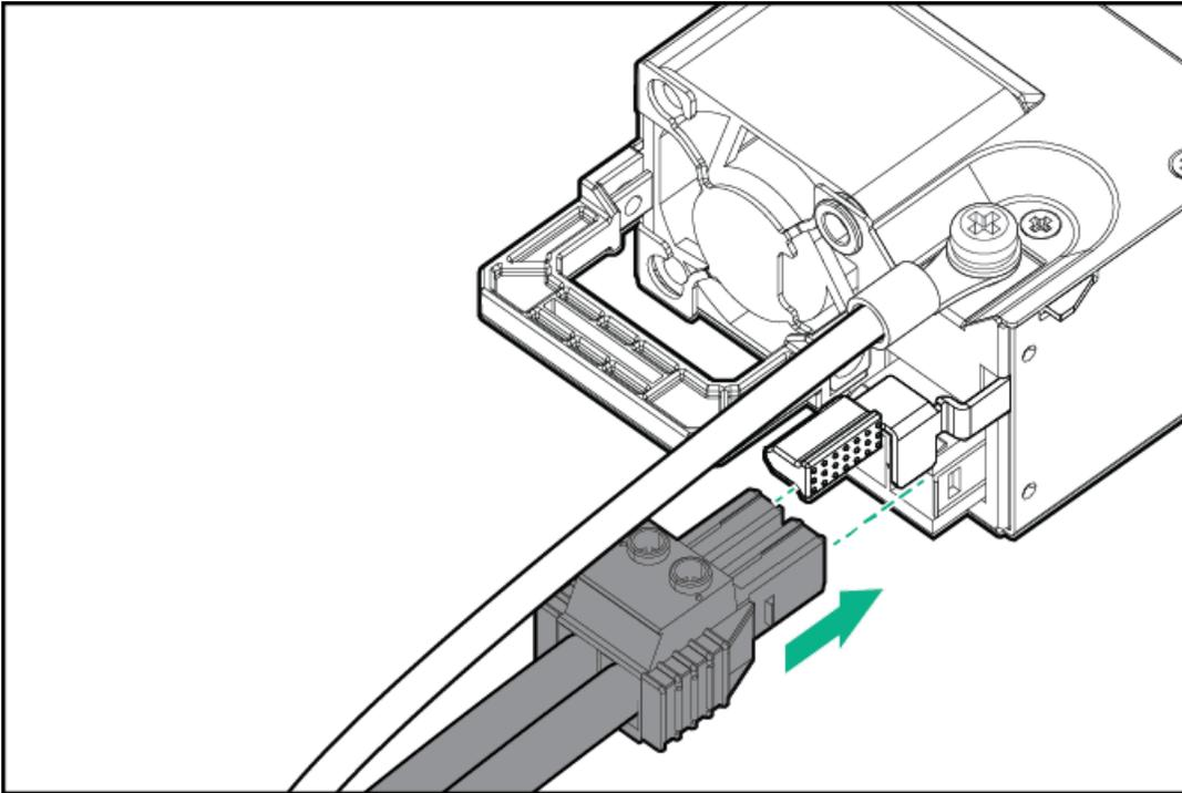
10. Secure the power cord, wires, and/or cables in the strain relief strap attached to the power supply handle:
