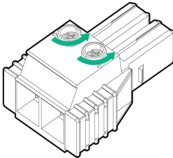
6. Attach the ground (earthed) wire to the ground screw and washer and tighten to 1.47 N m (13 lb-in) of torque. The ground wire must be connected before the -48 V wire and the return wire.
