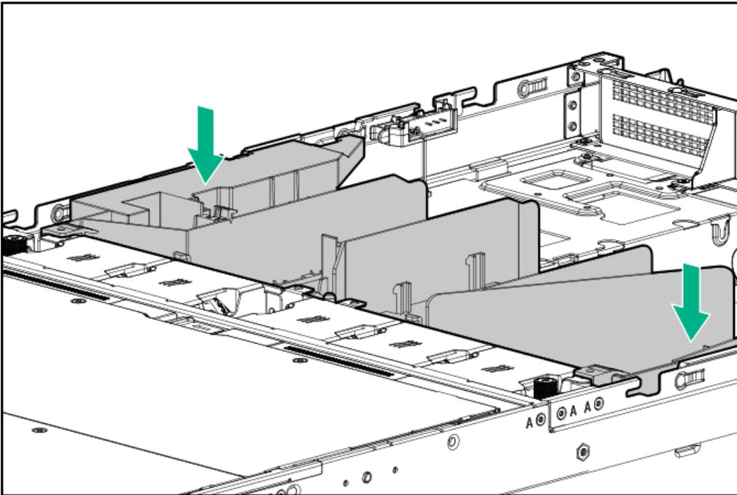
2. Install the performance air baffle.
