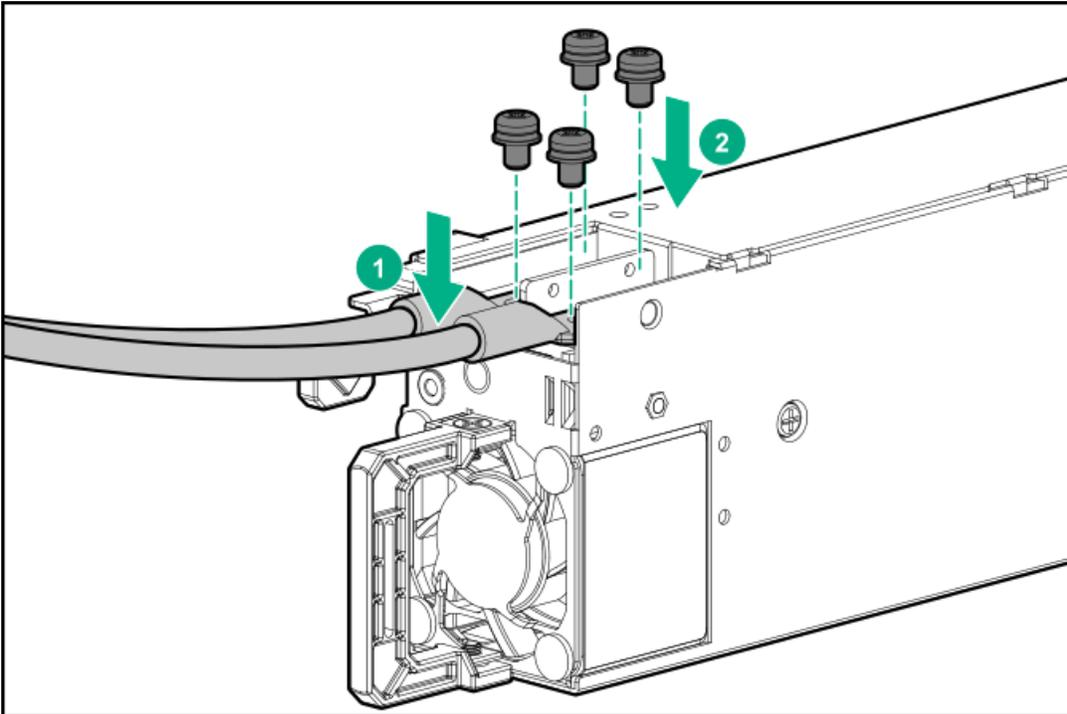
5. Attach the ground (earthed) wire to the ground screw and tighten to 1.47 N m (13 lb-in) of torque.
