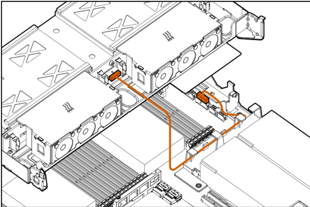
SFF drive cage 3 data cabling connected to the signal connector on the system board.
