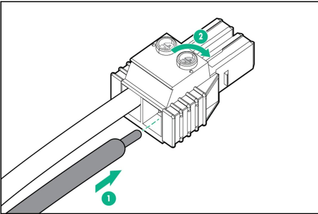
9. Install the terminal block connector into the power supply.
