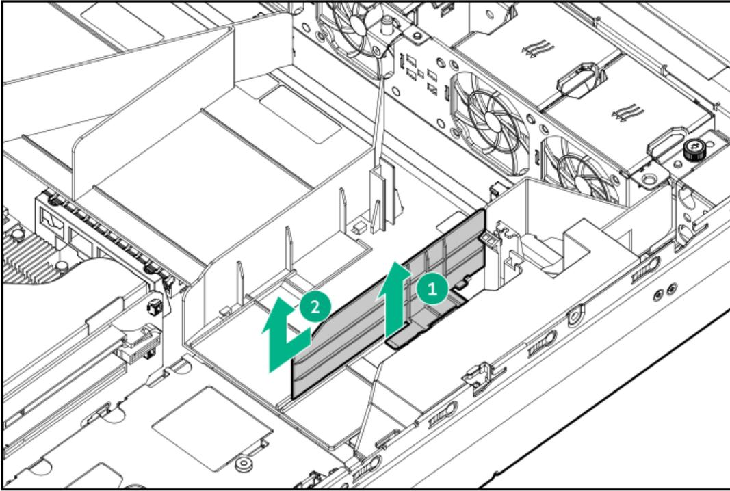
7. Reinsert the air baffle partition.
