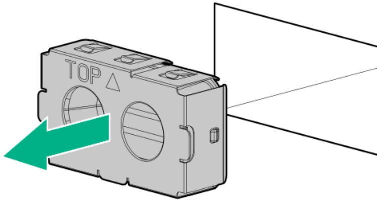
2. Remove the clear plastic cover on the side of the power supply.
