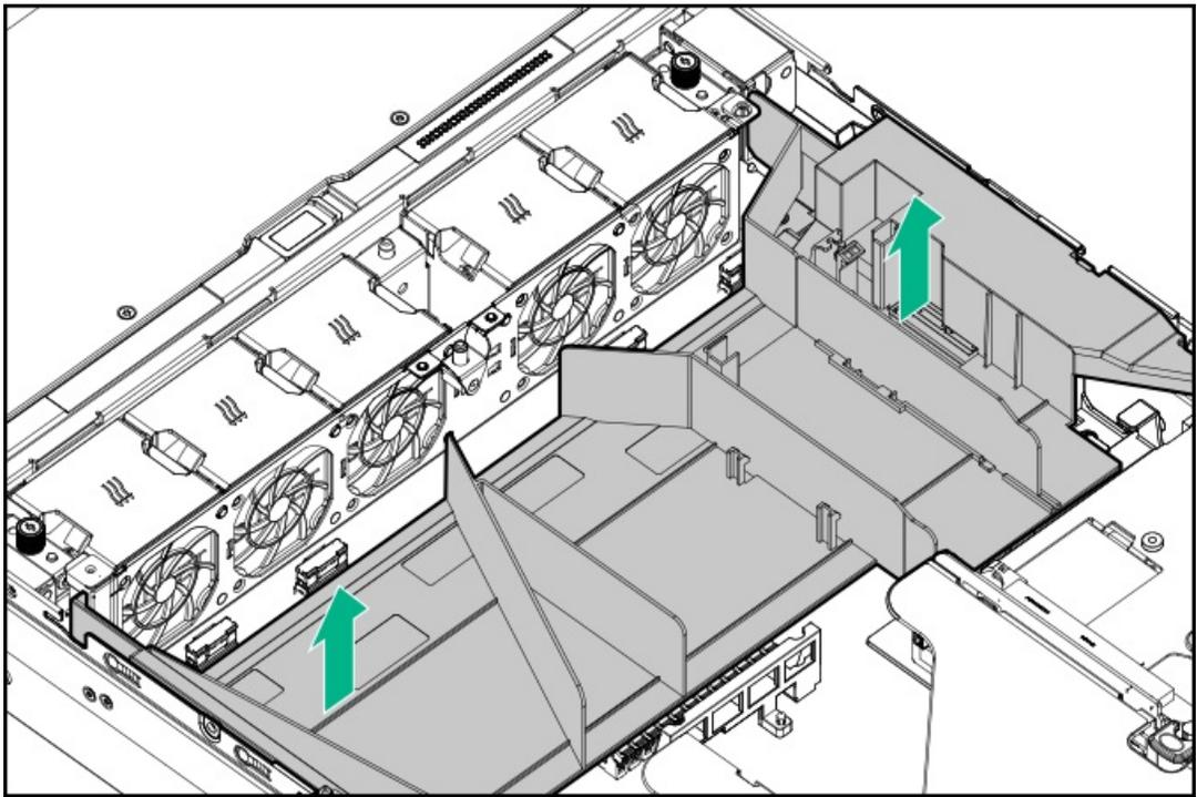
5. Remove the air baffle.
