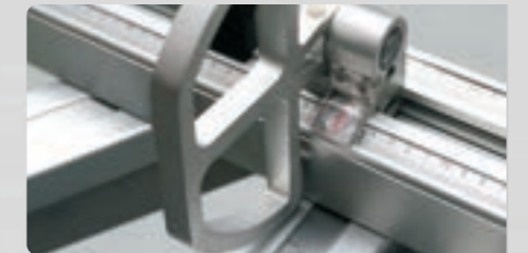
Large section profile cross cutting fence with reversible fence stops.
