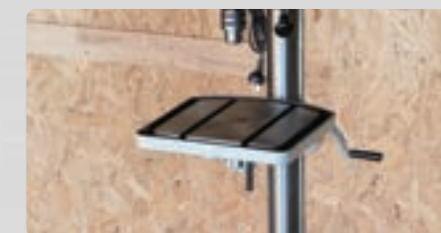
The cast iron, table has built in locating slots to allow for a vice to be securely held in place and can be tilted to allow for drilling at angles up to 45°.
