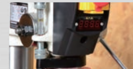
Set the depth adjustment knobs to limit your spindle travel for accurate and repeatable drilling operations.
