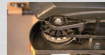
Mechanical variable speed drive system for easy speed changes from 400-2500rpm with the simple turn of the speed adjustment lever.
