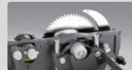
The saw unit is mounted on dual vertical shafts for smooth and accurate movement.
