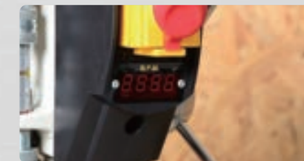
Digital read-out accurately displays current spindle speed.
