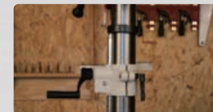
The table height is adjusted by a smooth rack and pinion system, makes adjustment easy.
