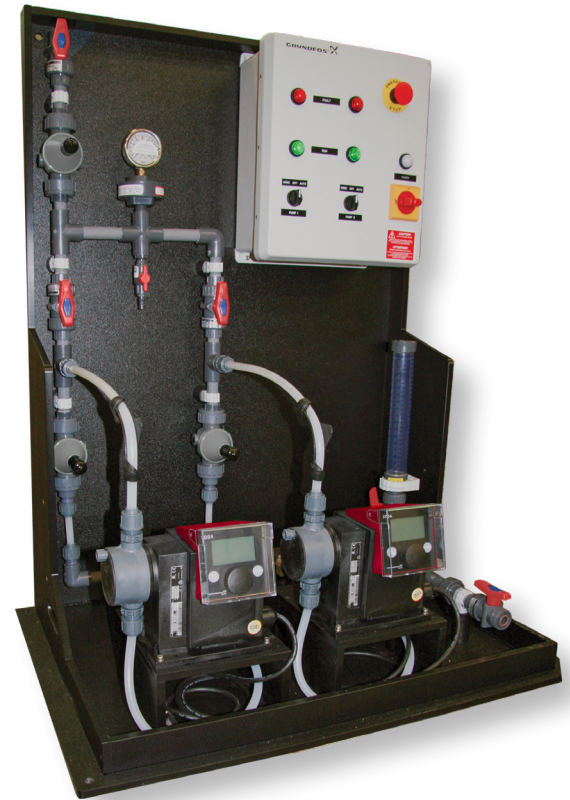
The DSS is a pre-engineered floor or panel dosing system package that offers integrated controls and one, two or three pump configurations designed to accurately meter liquid chemicals for a variety of water supply/treatment systems, as well as industrial and manufacturing applications. At the heart of each DSS, are the Grundfos SMART Digital Dosing Pumps.
