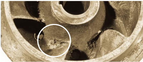
Cavitation corrosion of bronze impeller
