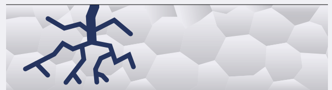
Fig. 1.6.10: Stress corrosion cracking
