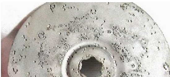
Pitting corrosion of EN 1.4401 (AISI 316)
