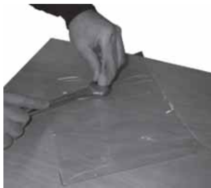
Fig. 45 Replacing the volume compensation bag
