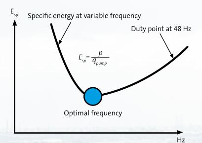
For energy optimisation, one of the important parameters to look at is the specific energy [Wh/m³]. Lowering speed in the system reduces dynamic friction in the pipes, and energy optimization can do this by ensuring the pump runs at the lowest possible speed without risk of sedimentation or blocking in the pump, pipes or pit.
