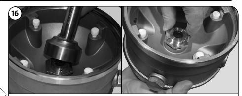
Flip the Pump Head Cover over to remove Shaft Seal (Pos. 105b). Using 00SV2107 or 41 mm Deep Socket, loosen and unscrew the Shaft Seal.
