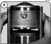
Remove the Cool-Top® assembly/Pump Head Cover (Pos. 77a). Light blows with a rubber mallet may be required to loosen assembly.
