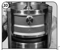
Remove the Pump Head Cover (Pos. 77a). Light blows with a rubber mallet may be required to loosen assembly.
