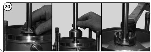
Slide the Inboard Seal (Pos. 105b) down the shaft and thread into the pump head. Use specialty tool, 005V2107, a 41 mm Deep Socket, or an Open Ring Spanner to torque the Inboard Seal to 26 ft.-lbs./35 Nm.
