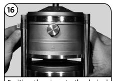
Position the plugs to the desired location; lower the completed Cool-Top® Pump Head Assembly (Pos. 77a) over the Shaft and seat on the Sleeve (Pos. 55). If it does not freely seat onto the Sleeve, STOP. Remove the Pump Head and turn over. Remove sleeve O-ring and stretch. Replace and reinstall the Pump Head onto Shaft and Sleeve. Skip to step 22.
