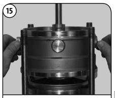
Remove the Pump Head Cover (Pos. 77a). Light blows with a rubber mallet may be required to loosen assembly.
