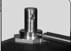
Pushing down on Shaft Seal collar (do not push down on Hex Nut), lower the new Shaft Seal (Pos. 105) over the Shaft. Use specialty tool, 00SV2107, a 41 mm Deep Socket, or an Open Ring Spanner to tighten to 26 ft.-lbs. or 35 Nm. Push the Shaft all the way down (for Tandem Seal models you must continue to apply downward force), then tighten the three 2.5 mm Shaft Seal Securing Allen Screws torque to 2 ft.-lbs. or 2.5 Nm.
