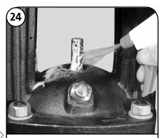
Spray soapy water onto the Seal O-ring Seating Surface of the Pump Head and the Shaft (Pos. 51). (If reusing original Shaft, be sure to use Emery tool provided with Seal Kit to remove any burrs on the Shaft. Then, spray with soapy water.)
