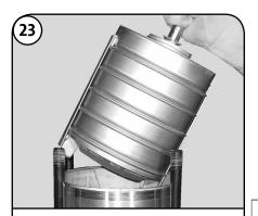
Grab the shaft and lift impeller stack out of the pump. If it is stuck, a light blow with a rubber mallet may be needed to jolt the stack free.
