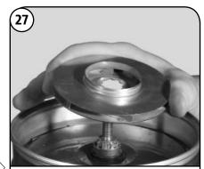
Lift the Impeller (Pos. 49a) off the shaft. If it comes off freely, proceed to step 29. If it is stuck and cannot be removed by hand, proceed to step 28.
