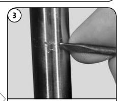
Before reusing the original Shaft (Pos. 51), use a light grit emery cloth to smooth away old set screw marks, as these can cut the O-rings in the seal assembly.
