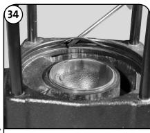
Remove, Sleeve O-rings (Pos. 37) in the Motor Stool (Pos. 2) or Pump Head (Pos. 77) and the Pump Housing (Pos. 6).
