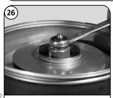
Using a 13 mm wrench, remove the Shaft Lock Nut (Pos. 67), Lock Washer (Pos. 66) and Splined Spacer (Pos. 64c).
