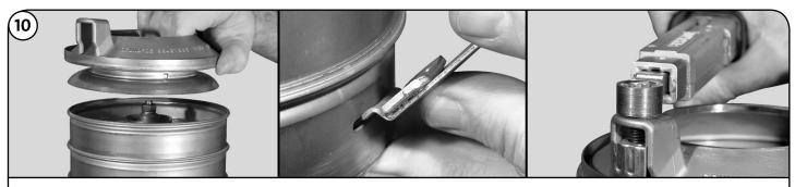
Place Suction Inlet Connector (Pos. 44a & b) onto Stack. Insert Straps (Pos. 26a) into slot in Top Chamber (Pos. 3). Place Washers (Pos. 26c) and Strap Bolt (Pos. 26b) on/into the Straps using a 13 mm Socket, 00SV0091, and Torque Wrench, 00SV0292, with Ratchet, 00SV0295, to Torque Bolt to 11 ft.-lbs./15 Nm.
