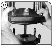
${\sf Spray}\, {\sf soapy}\, {\sf water}\, {\sf on}\, {\sf the}\, {\sf Sleeve}\, {\sf O-rings}$ (Pos. 37) in the Motor Stool or CRI, CRN Pump Head. Then lower and fully press in place.
