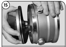
Press the plate firmly in place. Before proceeding to step 16, flip the Pump Head over; make sure the PTFE Stack "Compression Springs" (Pos. 60a) and the Sleeve O-ring (Pos. 37b) have been installed from step 1. If they have not been installed, follow the instructions in step 1 (page 9), then proceed to step 16.
