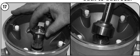
Insert Inboard Seal (Pos. 105b) into the bottom side of the prepped Pump Head Cover (Pos. 77a). Using the specialty tool, 00SV2107, or a 41 mm Deep Socket, tighten/torque seal the 26 ft.-lbs./35Nm.
