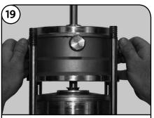
Position the plugs to the desired location. Lower the completed Pump Head Assembly (Pos. 77a) over the shaft and seat on the Sleeve (Pos. 55). If it does not freely seat onto the sleeve... **STOP**.
