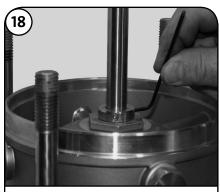
Loosen (approximately 1/2 to 1 turn) the three 2.5 mm Set Screws (Pos. 113) of the Inboard Seal (Pos. 105b).
