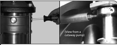
Loosen and remove the plug to allow access to Shaft Seal securing screw. Insert a 2.5 mm allen wrench to loosen (approximately 1/2 to 1 turn) the three Set Screws (Pos. 113) of the Inboard Seal (Pos. 105b).
