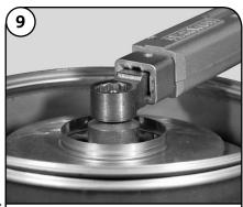
Lubricate the threaded end of the shaft with an FDA-approved lubricant. Thread the Lock Nut (Pos. 67) onto the shaft and torque to 16.3 ft.-lbs./22 Nm. Use 13 mm Socket, 00SV0091, Ratchet, 00SV0295, Torque Wrench, 00SV0269.
