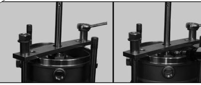
An alternative to step 21 is when the special tool 00SV2078 and two 27.5 mm Spacers (96491537) are used with two Staybolt Nuts and Washers.
