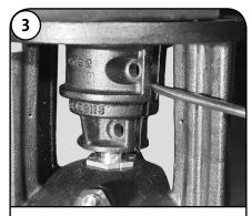
Remove Coupling Halves. Insert a slotted Screwdriver in Coupling gap and twist to free Coupling Half.
