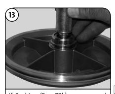
If Bushing (Pos. 79b) was removed from Disk Plate (Pos. 79a), use a Punch, 00SV2127, to install Bushing and Retaining Washer (Pos. 79c) into Disc Plate.
