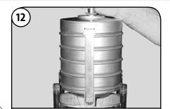
Lower new Stack Kit (Pos. 80) into the Pump Housing. Make sure it seats fully into the machined recess. (Chamber Straps must be located as pictured, 90° from suction/discharge ports).
