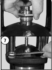
Remove the four 24 mm Staybolt Nuts (Pos. 36) and Washers (Pos. 66a).
