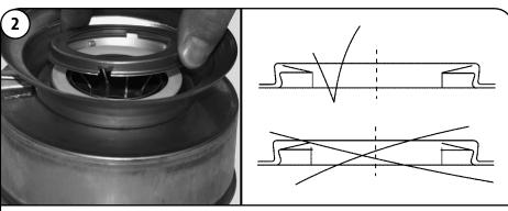
Replace any Seal Ring (Pos. 45) in the Chambers (Pos. 4, 4a, and 5a). Inner edge must face downward (see diagram). Snap Seal Ring Retainer (Pos. 65) into place. The retainer should not spin on the chamber, and the seal ring should move freely from side to side.
