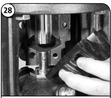
Install Coupling Halves (Pos. 10a). Spray a light machinery oil onto the Coupling Bolts (Pos. 9). Install loosely into the Couplings.
