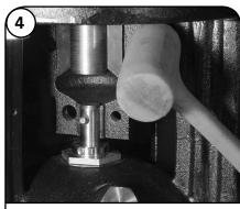
To free, remove remaining Coupling Half. Strike Coupling Half with a rubber mallet on upper edge. Remove shaft pin (Pos. 10).
