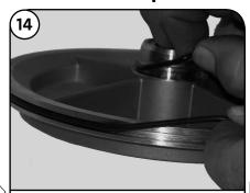
Place O-rings (Pos. 109a & 37c) onto the Disk Plate (Pos. 79a). Do not roll the O-rings; they should be stretched over and released into place to prevent cutting the material during installation into the housing. Spray soapy solution onto O-rings and housing.
