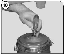
Before removing the Disk Plate (Pos. 79a) from the Pump Head (Pos. 77), inspect the Bushing (Pos. 79b). If worn, use a Flat Blade Punch or Special Punch, 00SV2127, and a mallet to drive out the Bushing.
