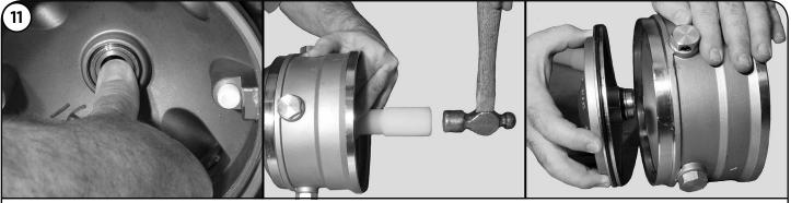
Remove the Disk Plate (Pos. 79a) from the Pump Head Cover (Pos. 77a) by pushing outward with your thumb. If stuck, use a Nylon Punch and a Mallet to drive out.
