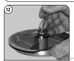
Remove the O-ring (Pos. 37c & 109a) from the Disk Plate (Pos. 79a).
