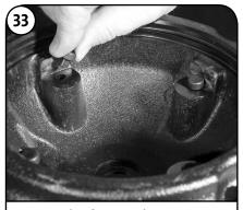
Remove the four Stack Compression Springs (Pos. 60) from the Motor Stool (Pos. 2) or Pump Head (Pos. 22).
