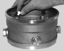
Remove the Sleeve O-Ring (Pos. 37) and the PTFE Stack Compression Springs (Pos. 60) from the Pump Head Cover (Pos. 77a).
