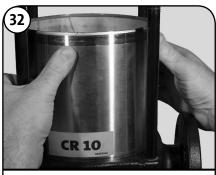
If the unit leaked around the Sleeve (Pos. 55), removal of the Sleeve may be required. Grip Staybolts (Pos. 26) diagonally. Using your thumbs, press against the Sleeve to release it from the Pump Housing (Pos. 6). Lift off sleeve. (Rocking or light upward blows with a rubber mallet may be required.)
