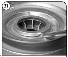
To remove Seal Ring (Pos. 45), insert a slotted screwdriver in relief slot of Seal Ring Retainer (Pos. 65) and twist or use Puller 00SV0239.
