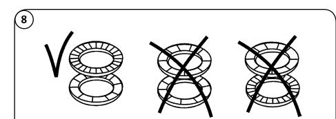
The Lock Washers (Pos. 66) come as a set. If they become separated, it is important the washers are repositioned correctly as noted in the diagram. The tabs should interlock while the serrated edges both point outward. Place the washers onto the shaft.
