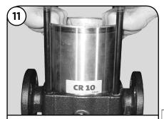
Spray soapy water on the Sleeve O-rings (Pos. 37). Then lower and press Sleeve (Pos. 55) firmly into place.
