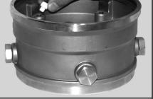
Remove Sleeve O-ring (Pos. 37) from the pump Head Cover (Pos. 77a). Then remove the PTFE Stack Compression Springs (Pos. 60a) from the Pump Head Cover.
