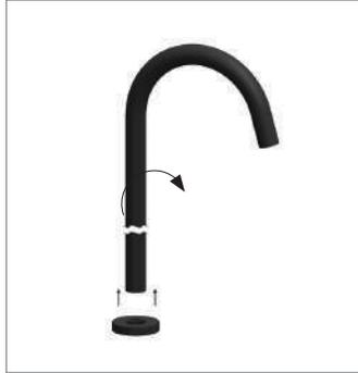
3. Position the spout outlet over the bath before tightening the grub screw.
