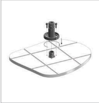
2. Slide the cover plate onto the spout from the bottom before fastening the spout to the base.
