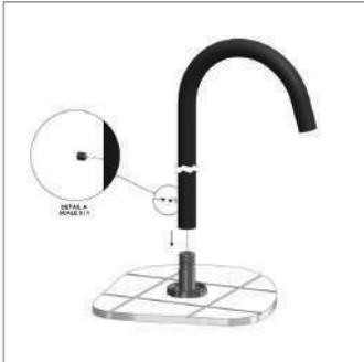
4. Slide the cover plate down over the base plate once the floor bolts have been tightened.
