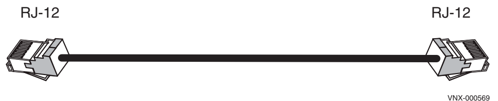
Figure 17 Example of LCC (RJ-12) to SPS (RJ-12) cable
