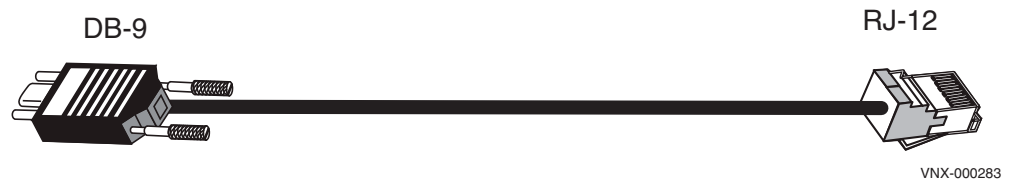
Figure 16 Example of SP management module (micro DB-9) SPS (RJ-12) cable
