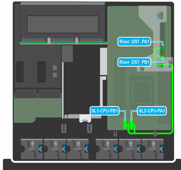
Figure 99. Riser 1A connecting on system board
