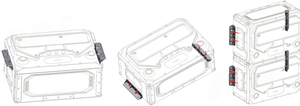
Figure 5-1: VRLV2560, 5120 batteries Installation Drawing
