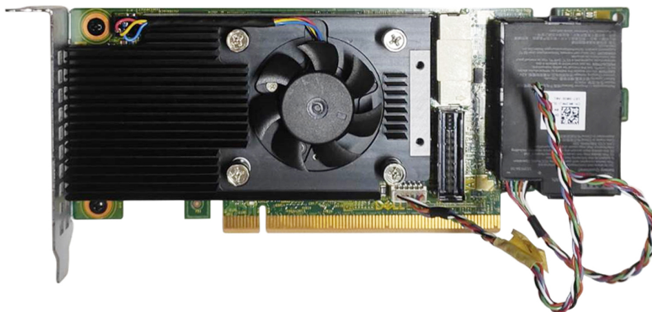
Figure 2. PERC H965i Adapter with a detachable battery
