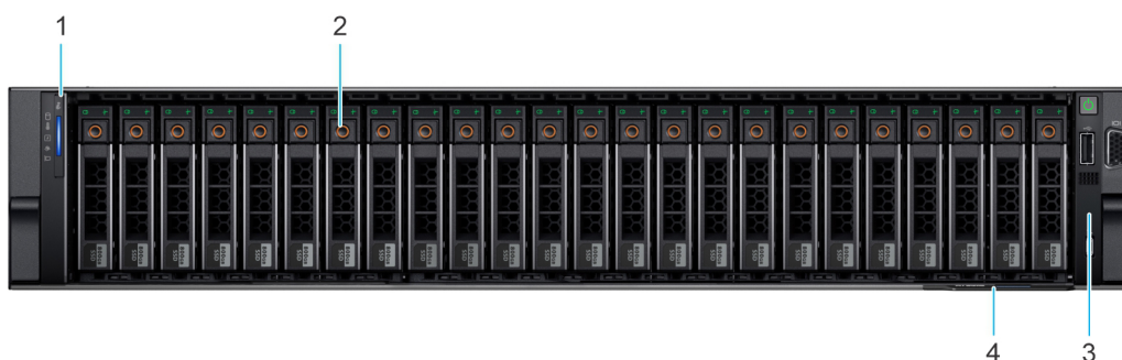
Figure 1. Front view of 24 x 2.5-inch drive system
