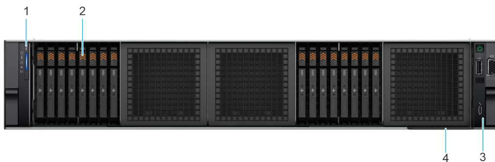
Figure 5. Front view of 16 x EDSFF E3.S drive system
