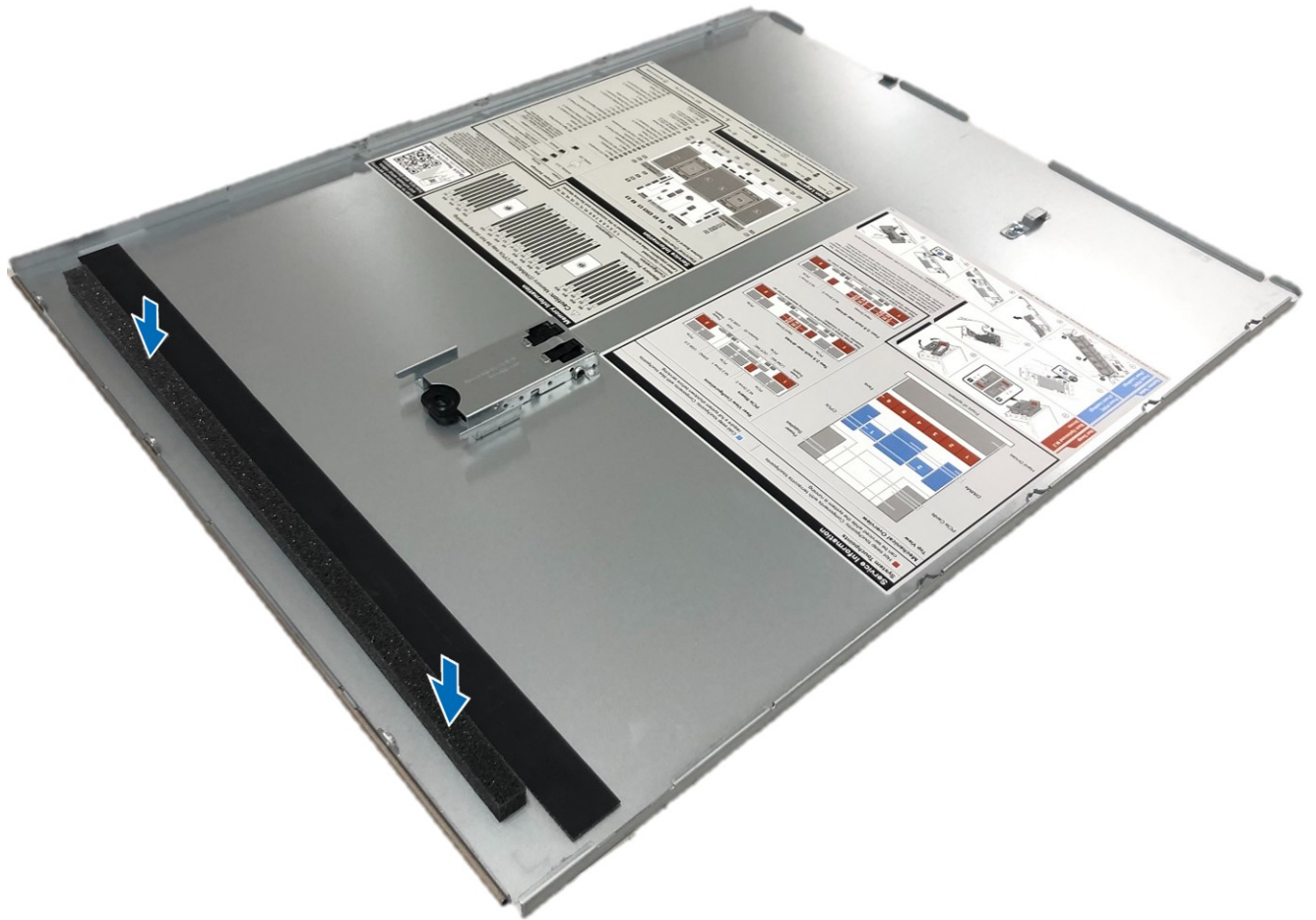
Figure 309. Installing foam on the system cover
