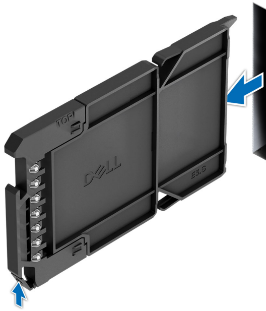
Figure 77. Removing an EDSFF E3.S drive blank
