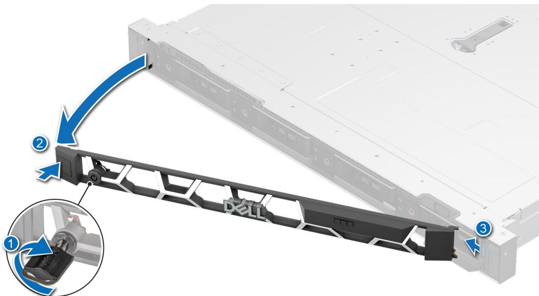
Figure 57. Removing the front bezel with the LCD panel
