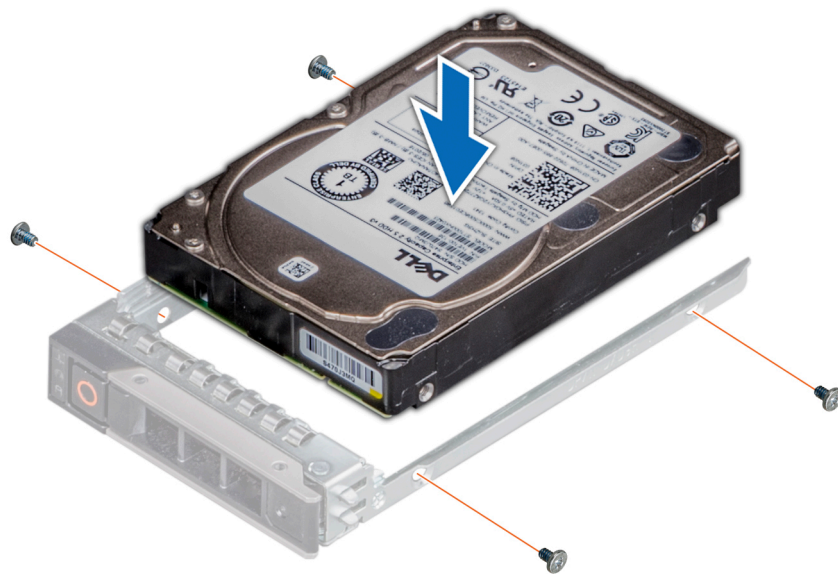
Figure 71. Installing a drive into the drive carrier
