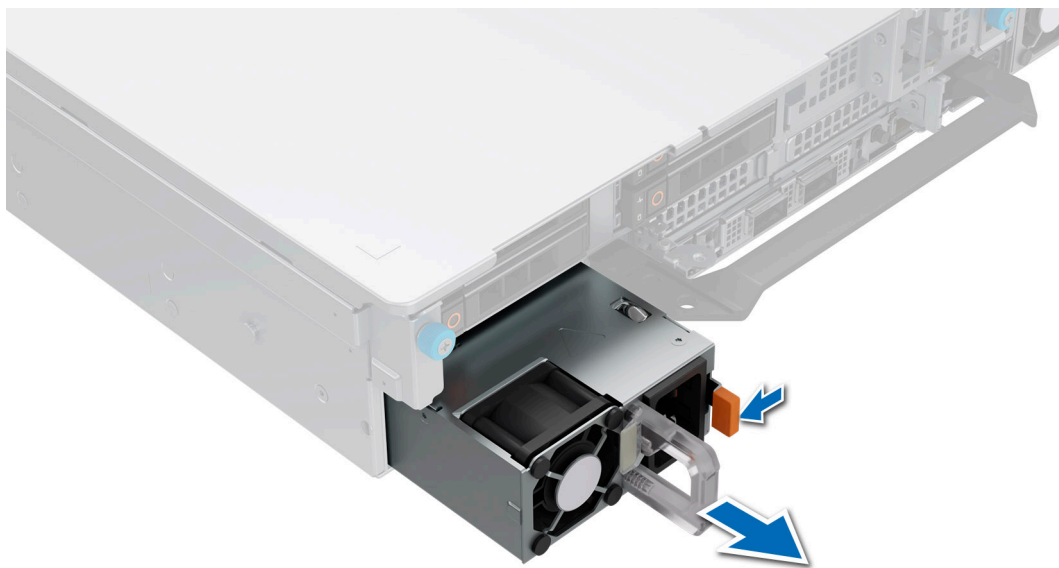
Figure 189. Removing a power supply unit
