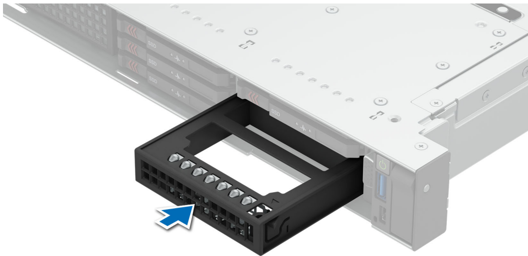
Figure 63. Installing a drive blank
