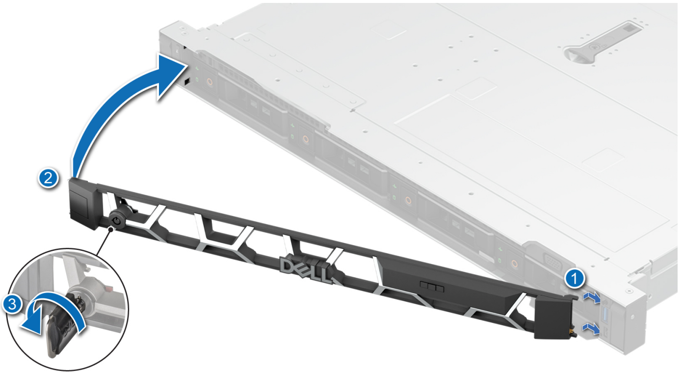
Figure 44. Installing the front bezel
