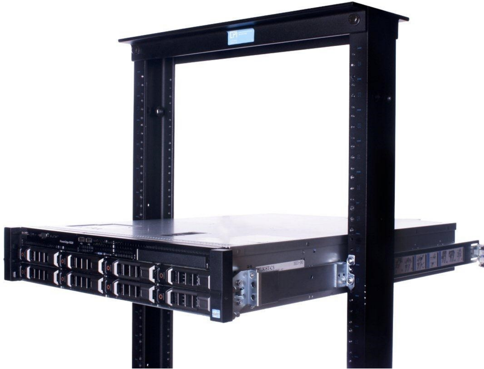
Figure 204. Static rails in 2-post center mount configuration
