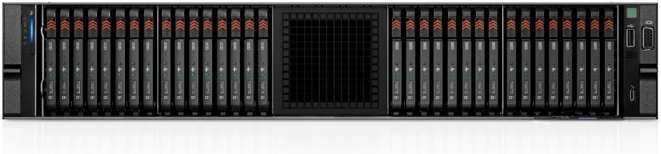
Figure 6. Front view of 32 x E3.S drive system
